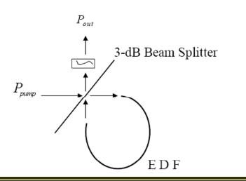
Γ(EDF confinement factor): 0.1 l (EDF length): 1m g (gain in EDF) =  $a(N - N_0)$ where  $a=10^{-24}$ m<sup>-2</sup>,  $N_0=10^{25}$ m<sup>-3</sup> η<sub>i</sub> (internal quantum efficiency in EDF): 1 α<sub>int</sub> (internal loss in EDF): 0 τ (carrier lifetime in EDF): 1 msec V = 10 - 10m3  $\lambda_{pump} = 0.98 \ \mu$ m
