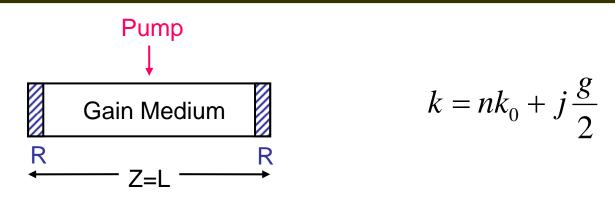
Assume there is an initial photon moving in z-direction inside gain medium.
